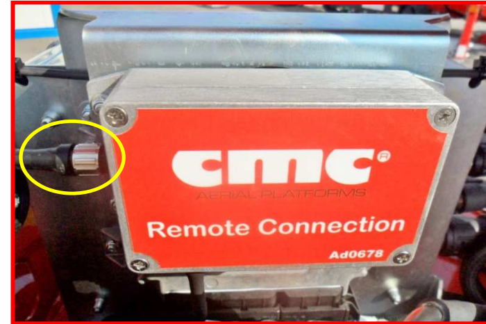
Picture 75: remote connection system.
