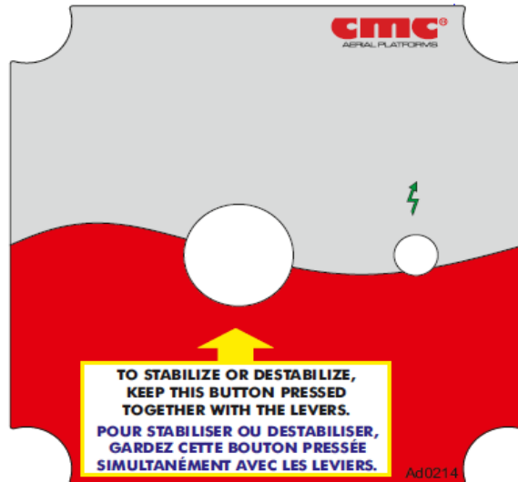
Picture 39: dead man box for stabilization/destabilization.
