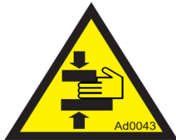
Picture 70: crushing and cutting hazard.
